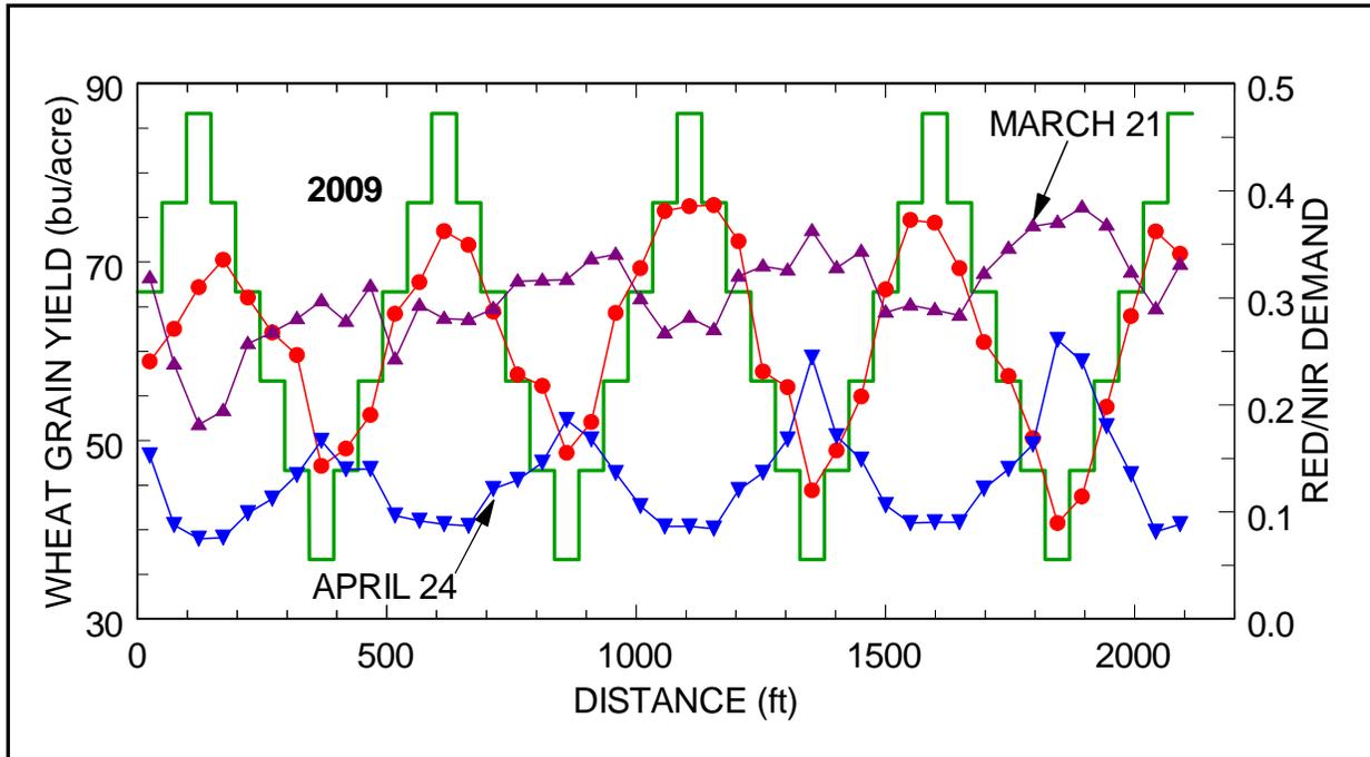
**Figure 3.** Wheat grain yield, nitrogen application rate and spatial pattern of nitrogen demand, reflected by the RIRR measurement at two different times.
