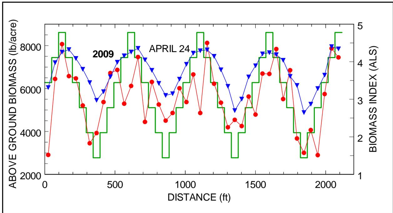
**Figure 5.** Biomass index measurements obtained with the ALS in comparison to hand-harvested aboveground biomass.
